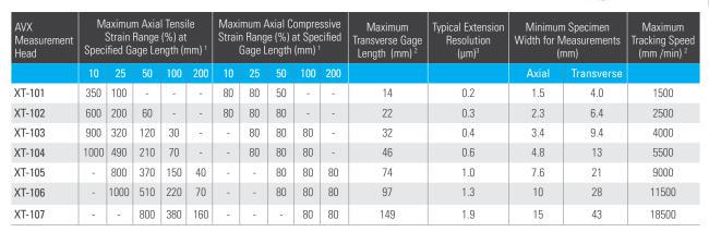
1. Strain ranges assume a distance between the grips of twice the GL, with a centrally positioned gage. Actual strain
